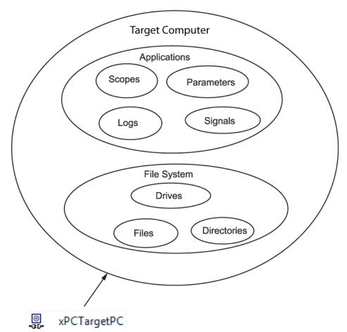
The API object hierarchy derived from the Simulink Real-Time system is shown in this conceptual diagram.
